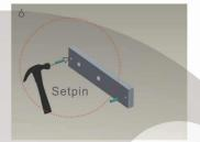
Strike the pin into the armature plate slightly (to avoid movement).
