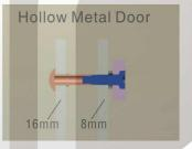
Drill a hole Inside: Diameter is 8mm Outside: Diameter is16mm
