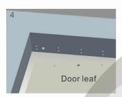
Drill holes based on the marked positions.
