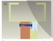
Close the door to test holding force. The angle between armature plate and magnetic lock can be adjusted by adding or reducing washers.
